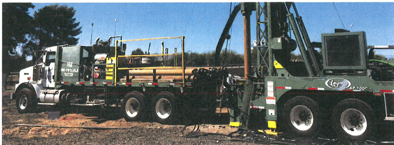
Drilling a groundwater monitoring well at a WQARF site.
